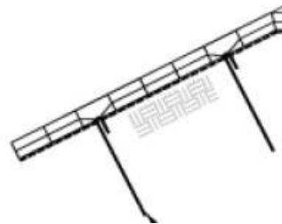
J HOOK ENGAGED TO TENDON FOR TENSION
