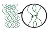
To create a strong seam, apply one staple per inch starting from top or bottom. A pneumatic stapler can be used for cell depths of 3" - 6". Or, we offer a hand-held stapler that can be used for the 3" - 4" cell depths.
